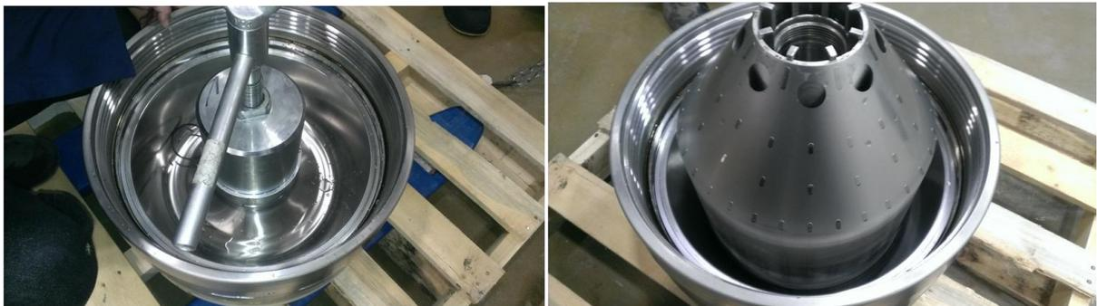
**Figure 3b.** Separator after cleaning cycle using 1.4 % OSA.
