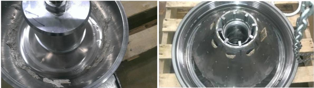
**Figure 3a.** Separator prior to cleaning cycle after 20 hours of production equivalent to 550K gallons of milk.
