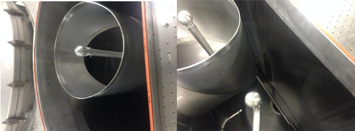
Figure 3a. Evaporator prior to CIP cycle after 30 hours of production equivalent to 670K gallons of milk.
