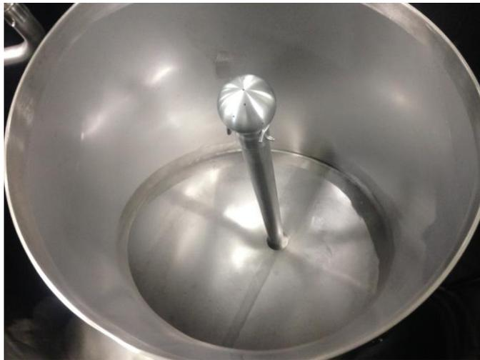
Figure 3b. Evaporator after CIP cycle using 1.8 – 2.2% OSAIk.
